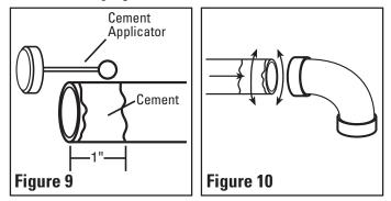
8. Insert tubing with cement into fitting with a twisting motion to ensure the cement has been evenly spread. Check that the tubing is evenly seated in the fitting and is aligned properly with the rest of the line (Figure 10).
